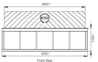
REMARKS - Above Dimensions are for 4000 mm Blocking Length and 800 mm Blocking Height:
