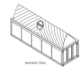
d- Blocking Height Intermediate Heights available from 500 to 1000 e- Case Width Typical for 800 mm Blocking Height (Changes Depending on Custom Blocking Heights)
